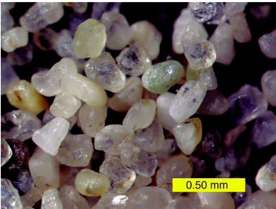
Sand seen under a microscope ("Mark A. Wilson", BY-SA license). Though smaller, the silt also appears as grains. Types of soils
